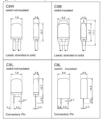
Standard leads: Stranded wires 0,50 mm²,100 or 300 mm long, Isolation Class B: colour yellow Isolation Class F and H: Colour white Stripped 5 mm
