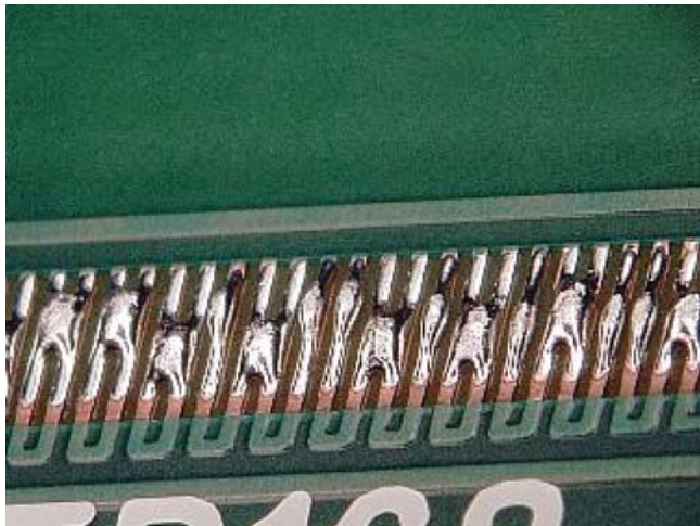
Figure 1-6 Bridging or Poorly Defined Solder Paste Printing
