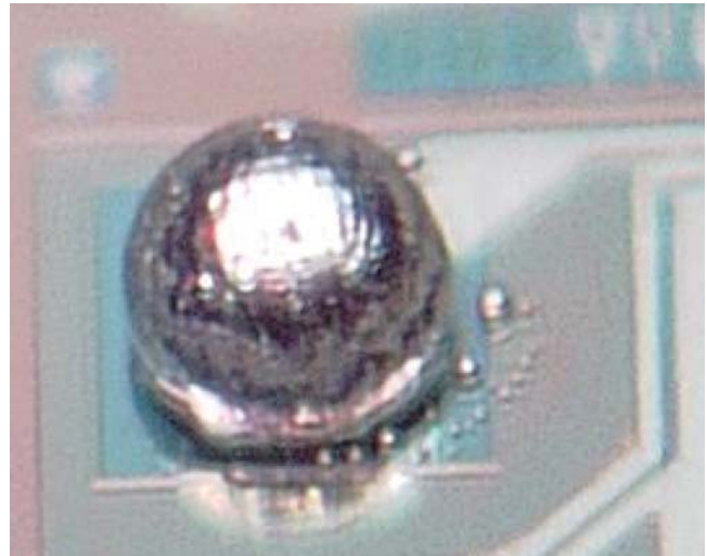
Figure 1-5 Solder Balls Following Solder Reflow
