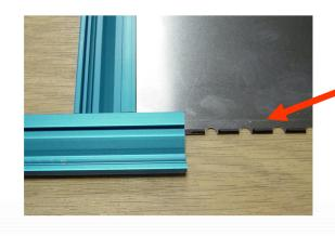
Metal on Metal connection for better tension, greater print area, and more consistent positional accuracy
